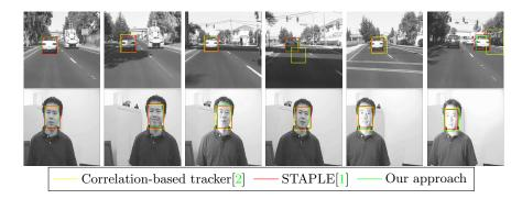
Fig. 8. Our tracking scheme is inherently robust to illumination changes because of the similarity measure we use in the localization step (4). The method performs comparable to STAPLE and outperforms the scale adaptive correlation tracker, which fails in the first sequence, in terms of accuracy.
