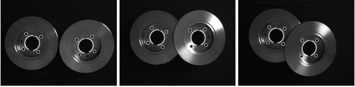
Figure 2. Two brake disks are detected despite partial polarity changes and perspective distortion. The illumination from the side creates specularities on the surface of the metallic object.
