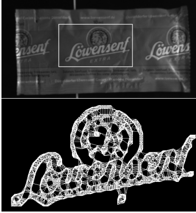
Figure 2: In the top image the rectangular white ROI defines the template. The bottom image depicts the extracted neighborhood graph of the model.
