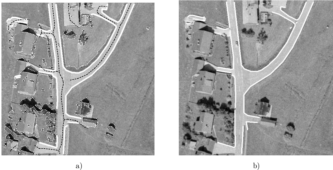
Figure 6: a) Input to the fusion process: hypotheses for road axes (dashed, black), hypotheses for road sides (solid, white) and other edges (dotted, white). b) Final road side hypotheses.
