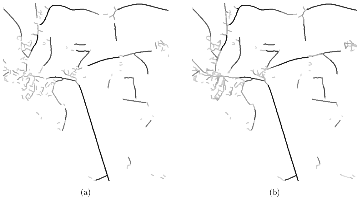
Figure 17: Weighted graph of road segments based on lines (a), with inserted connection hypotheses (b)
