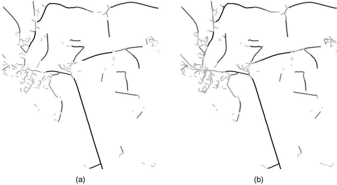
Figure 15: Weighted graph of road segments based on lines (a), with inserted connection hypotheses (b)
