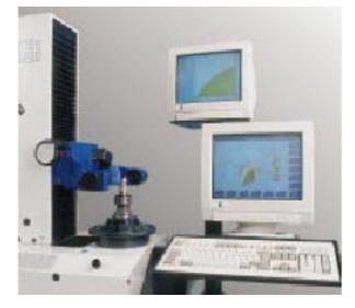
FIGURE 8: Machine for high precision measurements of tools with HALCON image processing
