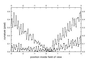
FIGURE 2: Curvature of a vertical line before (upper curve) and after (lower curve) calibration
