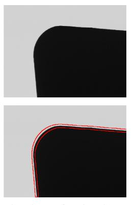
FIGURE 3: Image of a cutting tool (upper image) and region of interest for edge detection (lower image, red)
