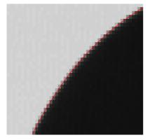
FIGURE 5: Edge of the cutting tool and subpixel precise edge (red line)
