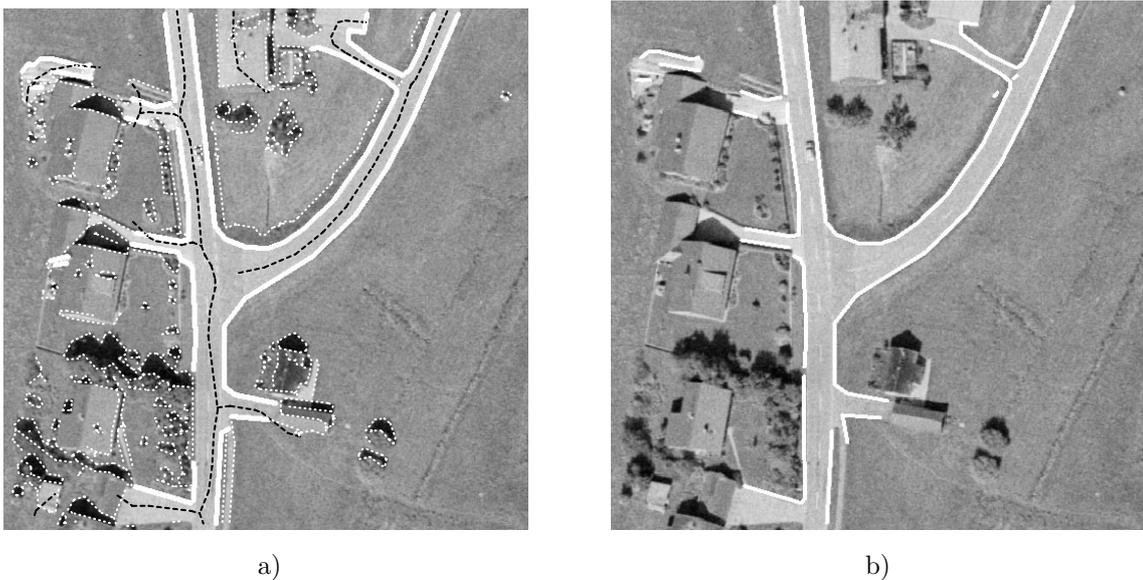
**Figure 7.** a) Input to the fusion process: hypotheses for road axes (dashed, black), hypotheses for roadsides (solid, white) and other edges (dotted, white). b) Final roadside hypotheses.
