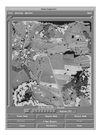
Figure 3: An inspector showing an image overlaid with regions resulting from a segmentation operation
