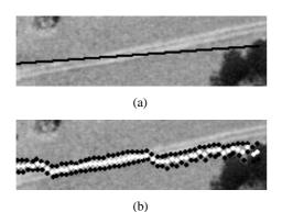
Figure 2: a) Inaccurate axis b) Skips in edge detection
