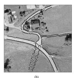
Figure 1: Edge points a) before and b) after the estimation of the road width
