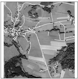
Fig. 2: Results of low resolution road extraction
